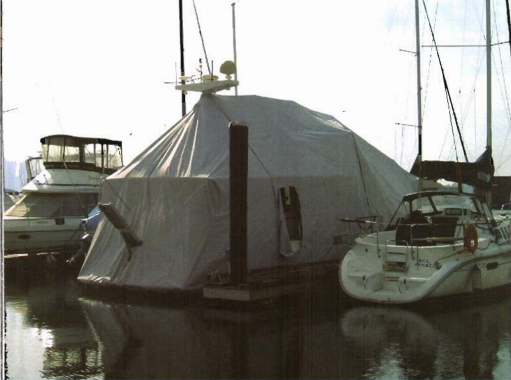
This Grand Banks 42 Europe is wrapped in a total winter cover with a five-foot width of 600-denier polyester fabric making up about 200 square yards. The cover consists of three parts with five supporting posts.
