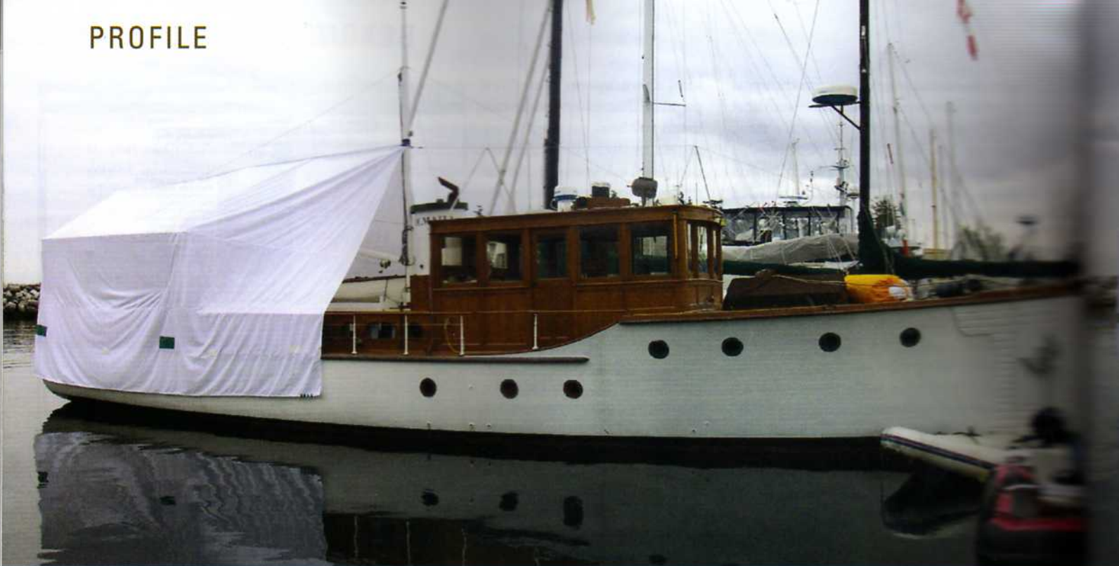
This Martinac boat was built in 1926 at the Martinac Boatyard in Tacoma, Wash. The four-part cover, completed in 2002, has approximately 180 yards of 5-foot-wide 600-denier polyester fabric. The opposite page shows the boat fully covered.
